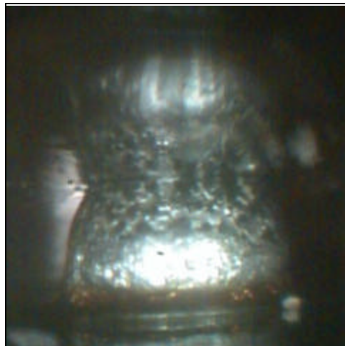
Excessive Flux left at the bottom of the solder ball after reflow
