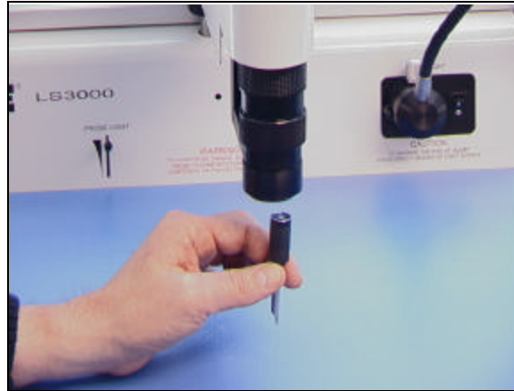
Figure 10. Installing the Rigid Probe
