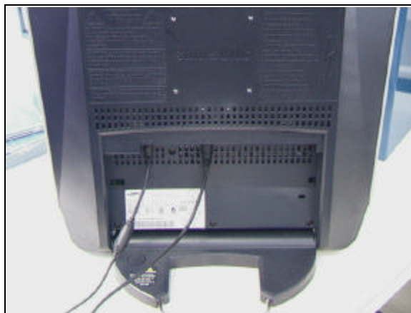
Figure 7. Power and Video Cables Attached to Back of Monitor
