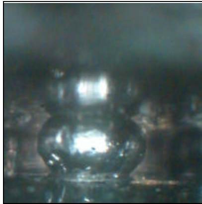
A good solder joint. Note the smooth shiny surface of the ball and good fillets on the top and bottom.
