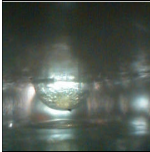
An open connection between the part and the PCB.
