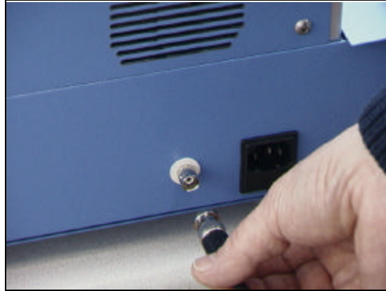
Figure 8. Attaching the Video cable to the LS 3000
