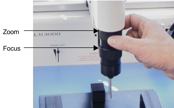
Figure 16. Focus and Zoom Adjustments
