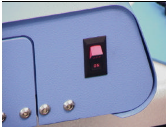
Figure 14. Main Power Switch in the On Position
